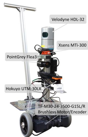
**Fig. 7.** The MinBot data collection platform and its sensor suite. Note we only use the Velodyne HDL-32 for detection and tracking. Also, only the motors' built-in encoders are used for additional robustness during localization and mapping.
