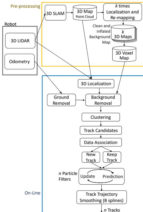
**Fig. 3.** Work flow of the dynamic object tracker. Both odometry and 3D lidar information is used from the robot. First using  $k$  data-collection runs in the environment, two maps of the static background are created, one for localization and one for background removal. After this pre-processing, we can localize, remove the static background, cluster the remaining points to detect and finally track a large number of dynamic objects on-line.
