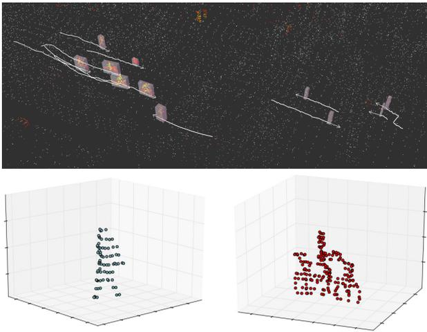
**Fig. 2.** Tracker output (top) at the Tsukuba Challenge. Dynamic objects are detected, with estimated bounding boxes and trajectory shown in white. Below, we show extracted, segmented pointclouds of a pedestrian (left) and cyclist (right).
